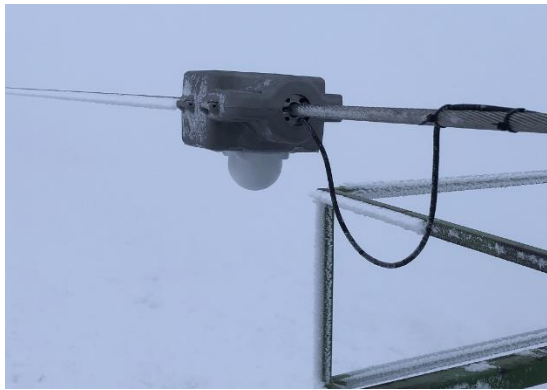
Fig. 10: Ampacimon™ vibration-based sensor [9] installed on single conductor (Conductor : ACSR LA-180, span length: 190 [m]) at Dead Water Fell test site (owner : EA Technology [21]) Sensor has been installed during a period with some deposit on conductor. Snow has been cleaned up close to sensor location for installation purpose (no snow in front of the sensor and snow behind sensor).
